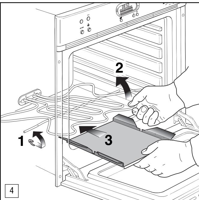
Position the pan support underneath the bottom heating element (fig. 4), than place the steamer on it with the lid on (fig. 5).
